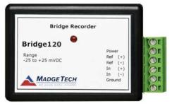
clock module. This easy-to-use device can measure and record up to 32,767 measurements per channel. The storage medium is non-volatile solid state memory, providing maximum data security even if the battery becomes discharged. The device can be started and stopped directly from your computer and its small size allows it to fit almost anywhere. The Bridge120 makes data retrieval quick and easy. Simply plug it into an empty COM or USB port and our user-friendly software does the rest.
