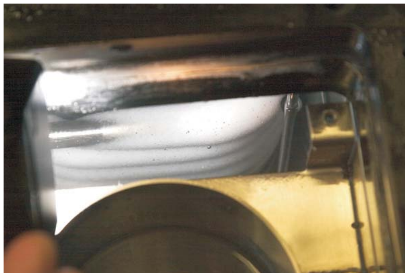
Figure 3 Cooling coil coated with ice. The fluid is pure methanol (no water added).
