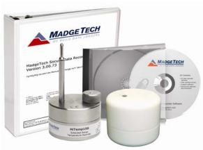
The HiTemp150 is completely submersible and can measure temperatures up to 150°C. The 2" rigid probe provides a fast response time and can record readings as fast as once per second. The HiTemp150 can be used in each autoclave cycle for verification and to provide data for validation. When used with the thermal shield the device can withstand up to 250°C (time dependent).
