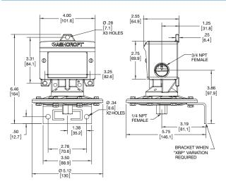
Differential pressure switch – psi differential ranges
