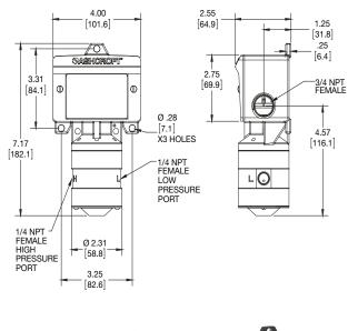
**Differential pressure switch – inches of water ranges**
