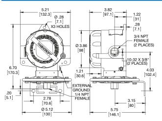
Differential pressure switch – psi differential ranges
