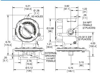
Differential pressure switch – psi differential ranges
