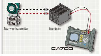
■ Input Command Check and Adjustment of Recorders and Controllers
