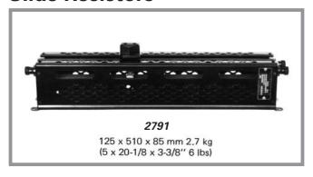
Model 2791 is composed of resistance wire with an insulating coating wound on a frame of special ceramic and a sliding brush that maintains contact with the wire. Resistance is continuously variable and can be increased or decreased as desired.
