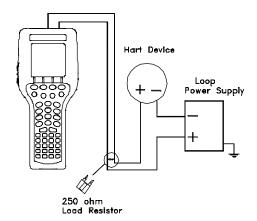
When connecting the YHC to a loop with a resistive load greater than 250  $\Omega$ s, the HART jacks may be connected across the loop + and – or to the HART device communication terminals. Refer to the following diagram for connecting across the loop + and -.
