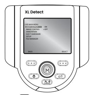
**Note:** Pressing the Freeze Frame key is a convenient way to temporarily turn off the light output and is ideal for changing optical tips and conserving battery charge.
