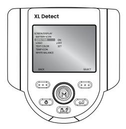
To change date format between MM/DD/YYYY and DD/MM/YYYY, select the Month, Day, Year format and move the joystick up or down to select prefered format. Select OK when finished.
