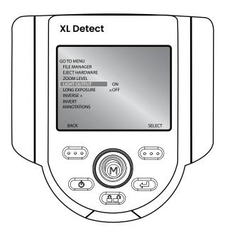
**Note:** Pressing the Freeze Frame key is a convenient way to temporarily turn off the light output and is ideal for changing optical tips and conserving battery charge.
