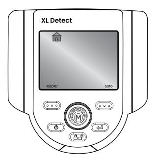
**Note:** It is recommended that a home operation is performed before withdrawing the camera from the asset being inspected, to avoid getting the camera stuck in the asset or damaging the XL Detect+.
