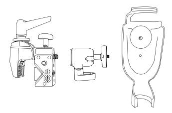
Secure the XL Detect+ mini magic clamp and place the XL Detect+ system in the handset holder.
