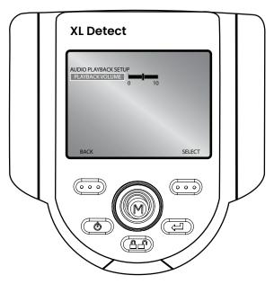
**Note:** XL Detect+ does not have a built in speaker, you must attach an external headset in order to playback audio annotation.
