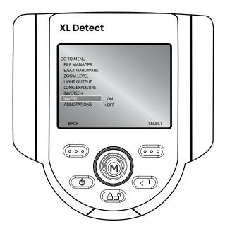
**Note:** Invert is typically used while a side view tip is installed in order to compensate for the inversion caused by this tip.
