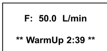
**Figure b-5:** XFM Main Screen during Sensor Warm up period.
