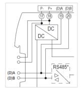
Figure 18 - RS485 TBUS terminal locations
