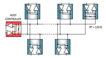
Figure 19 - Proper RS485 terminations
