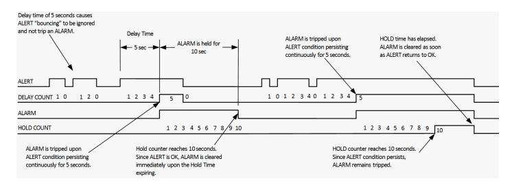
Figure 15 - Effect of Alarm Delay and Hold times on alarm behavior
