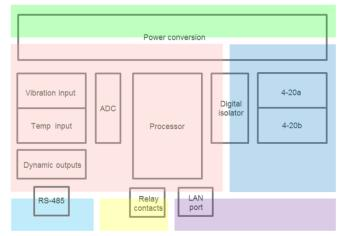
Figure 3 - Isolation diagram
