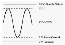
Figure 10 - Maximum input signal swing with 12V BOV
