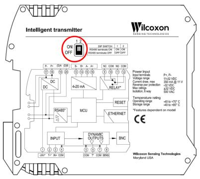
Figure 20 - RS485 termination DIP switch location
