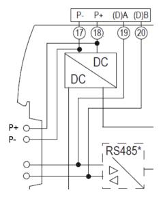
WARNING: The maximum current handling capacity of the power supply input terminals is 4 amps. When using these terminals to supply power to the TBUS, ensure the 4 amp rating is not exceeded.
