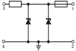
Figure 5: Typical zener safety barrier. The maximum end to end resistance (between 3 and 1) is 330  $\Omega$
