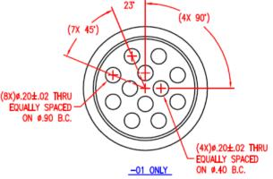
Figure 3: Cable feed through holes provided with cable grip option (12 hole)
