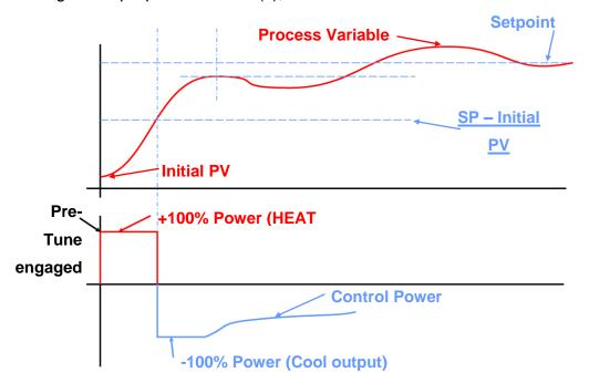
When Pre-Tune is completed, the PID control output power is applied using the calculated values. Pre-Tune limits the possibility of Setpoint overshoot when the controller is new or the application has been changed. It will automatically disengage once complete.
