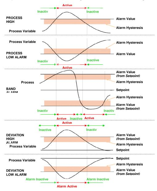
E.g. a high alarm's hysteresis band is below the high alarm value, and a low alarm's hysteresis is above the low alarm value. Also refer to *Alarm Operation*.
