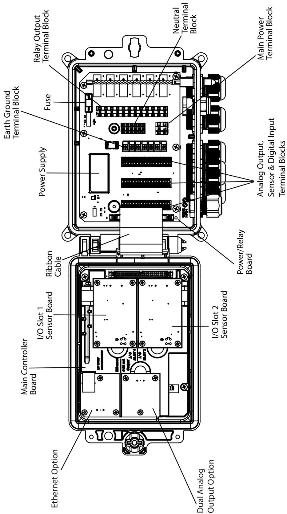
**Figure 6 Parts Identification**
