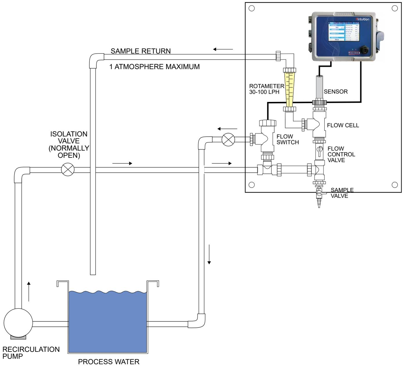
**Figure 3 Typical Installation – Disinfection Sensor**
