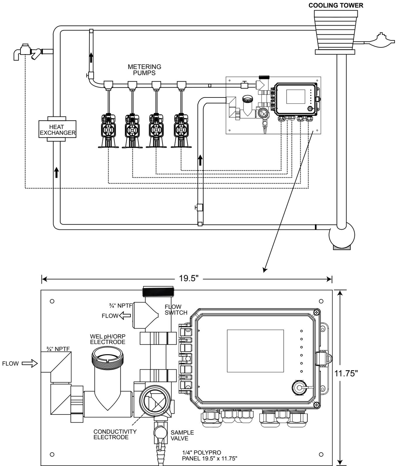
**Figure 1 Typical Installation – Cooling Tower**
