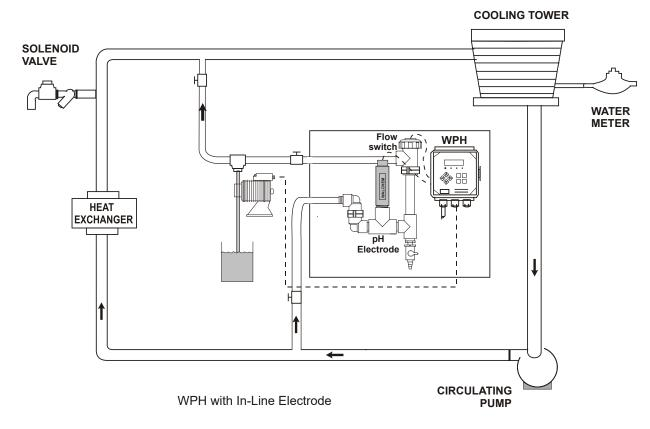
Figure 1 Typical Installation
