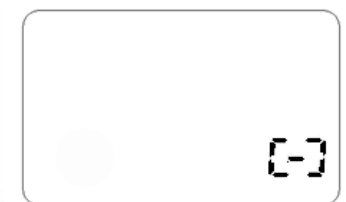
Meter Installed Backwards
