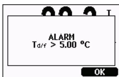
Figure 45 Display Alarm Active
