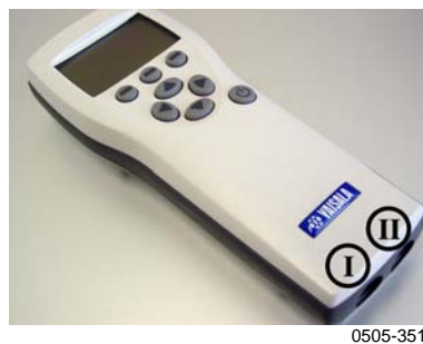
Figure 17 Location of the MI70 Probe and Cable Connector Ports
