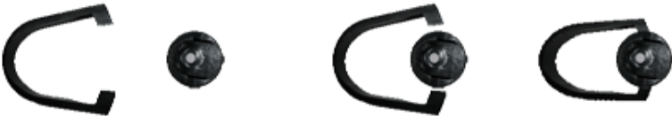
Figure 2. Using Electrode Stack Removal Tool
