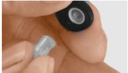
Figure 5. Inserting Lamp into Electrode Stack
