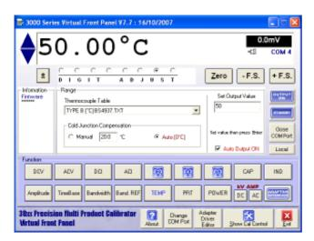
Using the Virtual Front Panel software from Transmille, custom configuration of temperature values can be achieved to any temperature standard providing the best flexibility.
