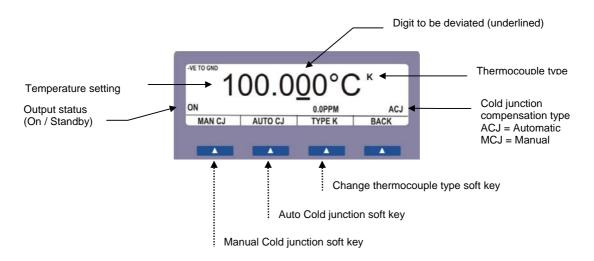
Once in thermocouple mode, the menus available at the bottom of the screen will change to reflect the thermocouple mode options - the available menu items are :
