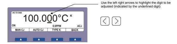
To increase or decrease the digit, simply use the up down keys on the calibrator's keyboard or use the digital potentiometer
