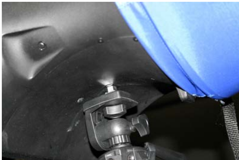
Figure 25: Mount Hood Base to Telescopic Stand
