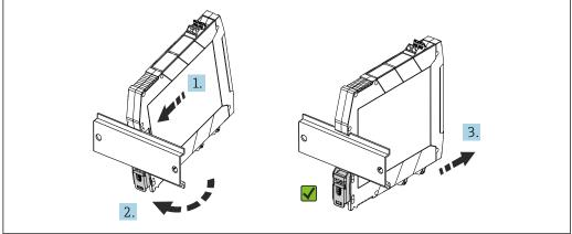
**№** 7 Mounting the DIN rail transmitter
