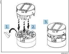
■ 15 Attach the display to the transmitter
