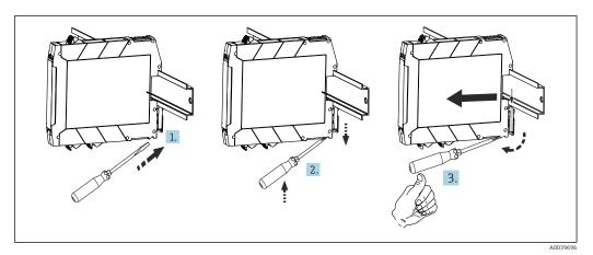
■ 8 Dismantling the DIN rail transmitter
