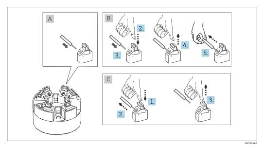
lacktriangledown 11 Push-in terminal connection, using the example of a head transmitter
