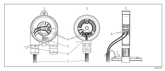
lacksquare 12 Connecting the signal cables and power supply
