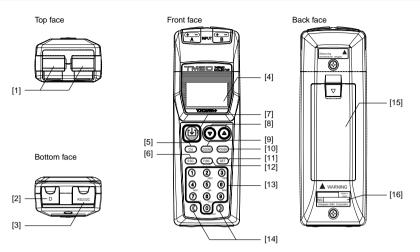
[1] External probe jacks (channels A and B) Used to plug in the cables of thermocouple type K, J, E, or T probes or voltage measurement (±100 mV or ±1 mV range) sensors. (A voltage measurement probe has a U-shaped omega connector.)
