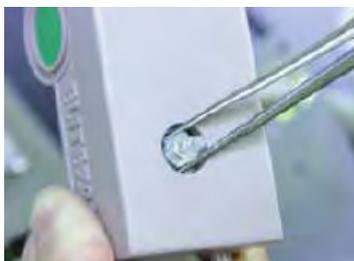
8. Slide the pump assembly out of the air pump body.
