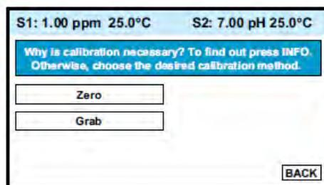
There are two steps to calibrating a free chlorine sensor, measuring the zero current (Zero) and determining the slope of the calibration curve (Grab). Because stable total chlorine standards do not exist, the sensor must be calibrated against the results of a laboratory test run on a grab sample.
