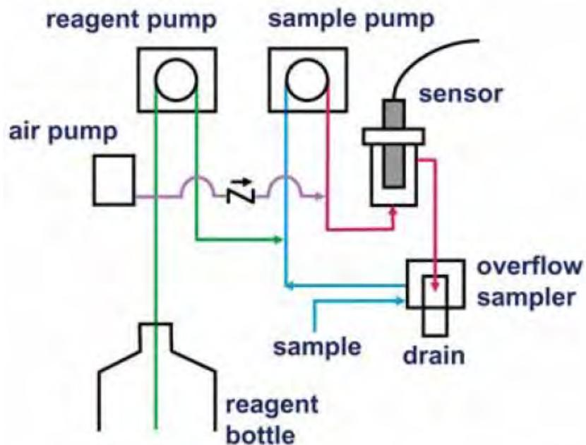
The treated sample next enters the flow cell. Bubbles injected into the flow cell produce turbulence, which improves the stability of the reading. A membrane-covered amperometric sensor in the flow cell measures the concentration of iodine. The transmitter receives the raw signal from the sensor and displays the concentration of total chlorine. Display units are ppm (mg/L) chlorine as  $\text{Cl}_2$ . The treated sample leaves the flow cell and drains to waste along with the excess sample.
