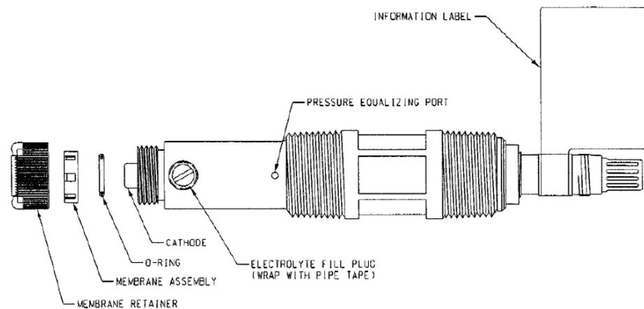
3. Hold the sensor over a container with the cathode pointing down.
