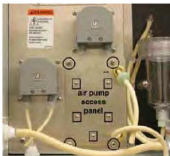
4. Disconnect the air inlet and outlet tubing from the air pump.
