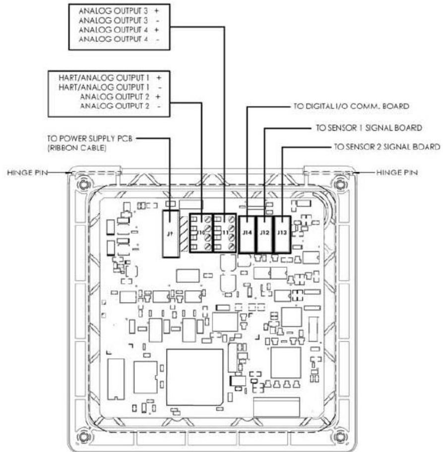
6. Slide the replacement board partially into the board slot. Plug the sensor board into the main board and reattach the sensor wires.
