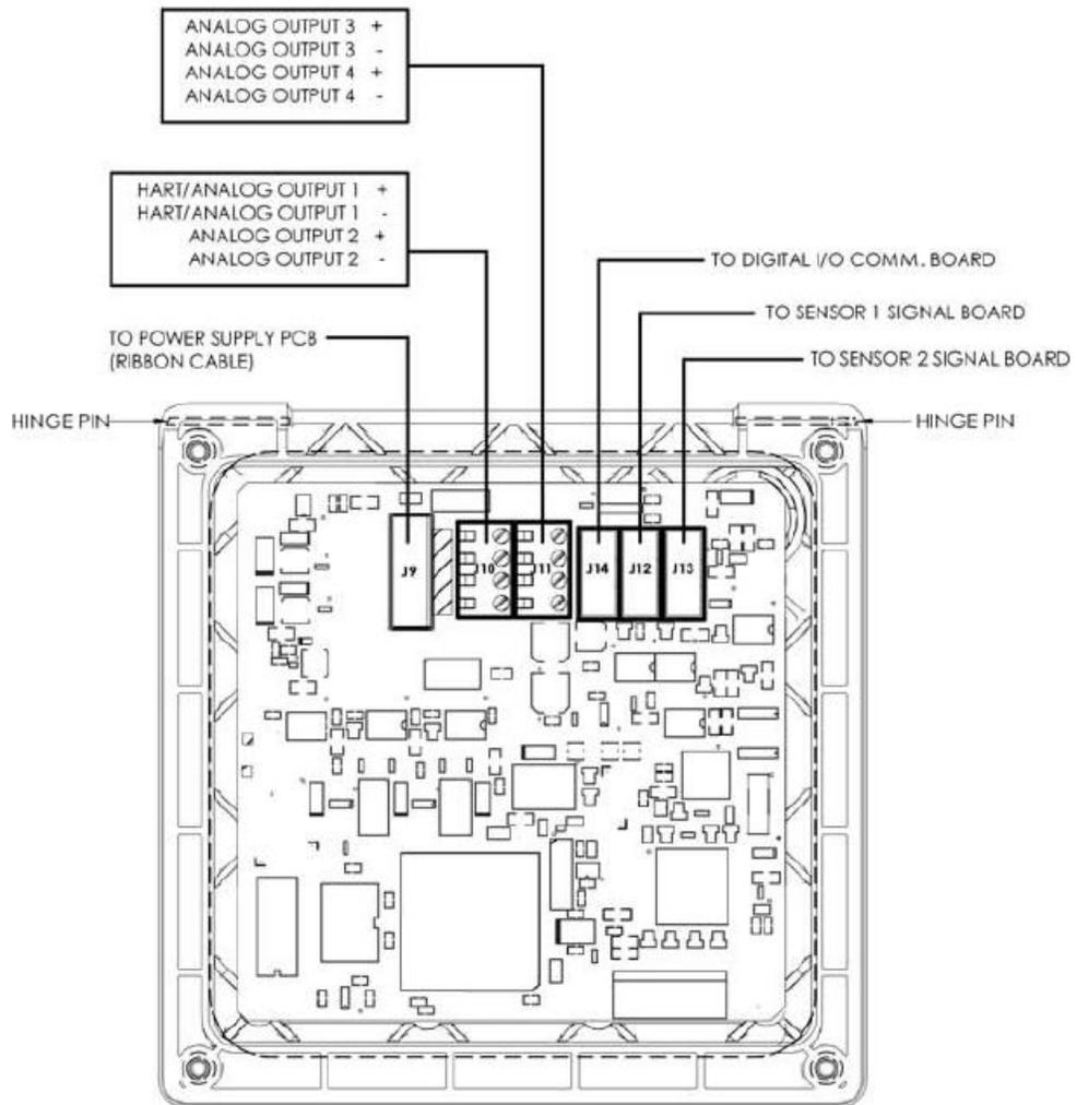
The analog outputs are on the main board near the hinged end of the enclosure door.
