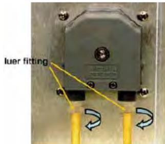
3. Using your thumb and forefinger, gently pinch the sides of the pump cover. Slide the cover upwards to remove it.
