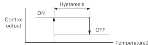
Ex)If temperature range is 0 to 400°C and hysteresis is 0.5%(2°C), therefore when the set value is 300°C, 301°C:OFF and 299°C:ON.
