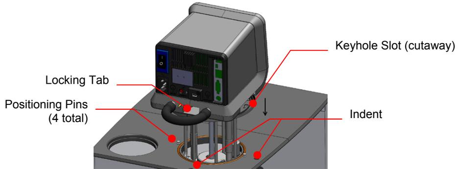
2. Gently rotate the Temperature Controller until it drops down on the positioning pins.
