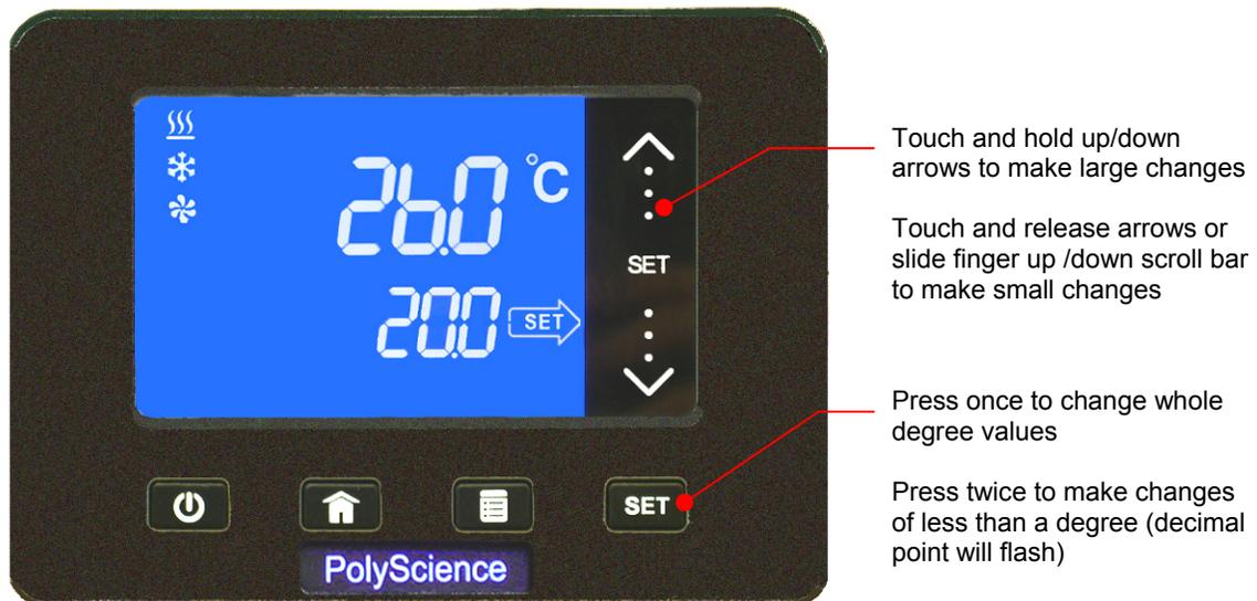
**To Change:** Press **SET**. The arrow around the word “SET” will begin flashing. To make changes of one degree or more, touch the up/down arrows until the desired set point temperature is displayed. To make changes of less than a degree, (e.g.,  $0.50^{\circ}\text{C}$ ), press **SET** a second time. The decimal point will begin flashing. Touch the up/down arrows until the desired value is displayed.
