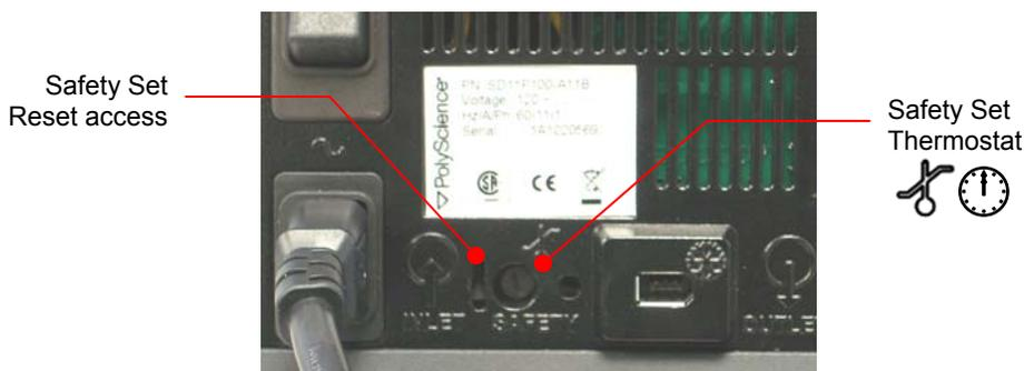
1. Using a small flat blade screwdriver, rotate the Safety Thermostat clockwise until it stops.
