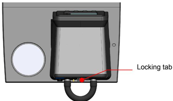
2. Rotate the Temperature Controller clockwise until it stops (about 0.75 inch / 1.9 cm).
