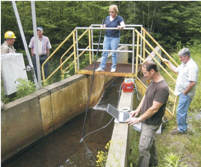
Stingray performance demonstration before installation in a 36" Parshall Flume
