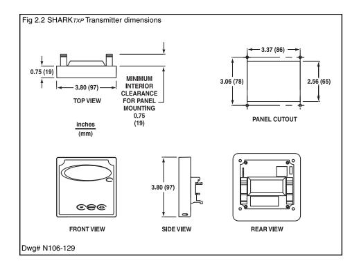
**Panel Mount** – The transmitters can be panel mounted to a panel using the hardware kit provided. The panel cutout dimensions are shown in fig. 2.1 and 2.2.
