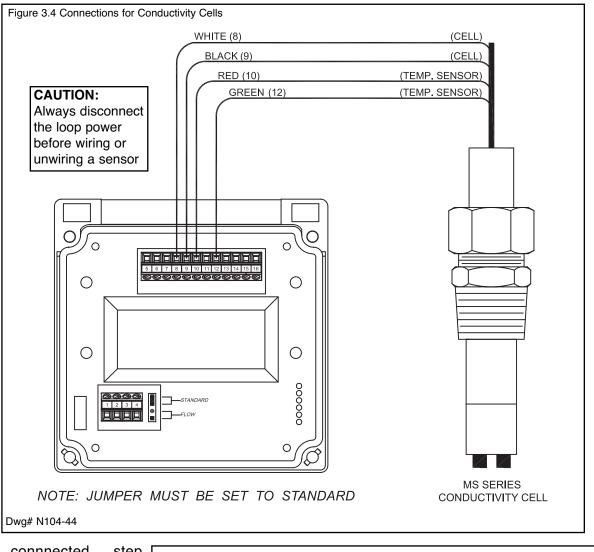
Once connected, step through the LCD menus to select the cell in the order shown. The TEMP COMP CURVE setup default is 1.8%/deg C. This is acceptable for most process applications. If your process is significantly different from this, change the setting in the TEMP COMP CURVE menu.
