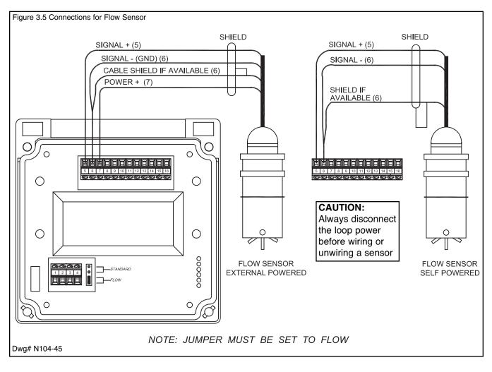
Once connected, step through the LCD menus to select the sensor in the order shown. The Sensor K factor (pulses per U.S. Gallon) is usually printed on the side of the sensor or on a label attached to the sensor cable.
