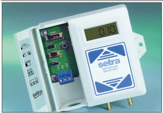
ers sense differential or gauge (static) pressure and convert this pressure difference to a proportional electrical output for either field selectable unidirectional or bidirectional pressure ranges. The 260 Series is offered with field selectable high level analog outputs of 0 to 5, and 0 to 10 VDC, or 4 to 20 mA.
