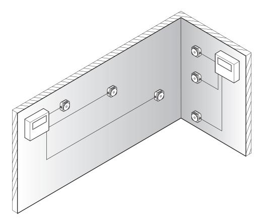
A gas detector system uses analog current loop principle. Each detector is individually wired to the controller on its own cable.
