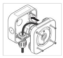
7. Remove power and refit the detector module to the back box.
