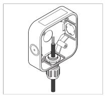
2. Feed the cable through the cable gland.
