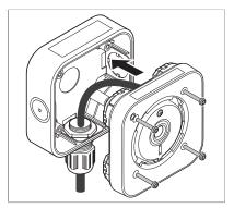
2. Position the detector module onto the back box ensuring that the status indicator is in the top left-hand corner when viewed from the front. Tighten the four retaining screws using a No. 2 Phillips screwdriver to secure.
