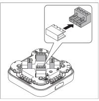
3. Turn over the detector module and locate the terminal blocks on the back. Remove the terminal blocks by pulling them toward the center of the module.
