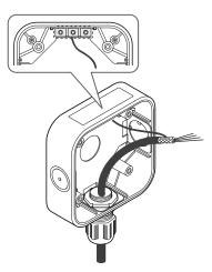
Effective grounding is crucial to ensure stable communications and to limit the effects of radio frequency interference. Ground points are provided inside the back box. In order to prevent false readings or alarms as a result of ground loops, ensure that the shield of all cables are grounded at a single point, preferably at the controller. Consideration should also be given to how conduit, glands and the internal earth plate are also grounded.
