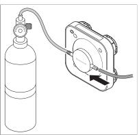
4. Connect another tube to the other gassing port, and place the end of this tube in a position so that gas can exhaust safely away from the work area and other personnel.
