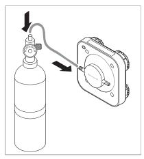
3. Connect a tube from a cylinder of calibration gas to either of the cap's gassing ports.
