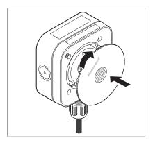
4. Replace the front cover. Place the front cover into the detector module in the position shown and rotate it clockwise until it locks into position.
