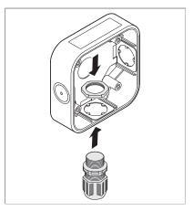
Fit suitable cable glands appropriate to the application and type of cable being utilized to the opened cable entries.
