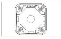
1. There are four screw positions in the rear of the back box for mounting purposes. Punch the required screw positions or drill using a 4 mm drill.
