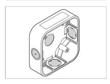
3. There are four cable entry knock-outs on three sides of and on the rear face of the back box. Drill or punch the entries as required.
