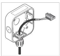
4. Connect the cable to the appropriate terminal block, referring to the relevant wiring diagram. Strip and insert the end of each wire into the corresponding terminal hole. Using a flat-blade terminal screwdriver, tighten the terminal screw until the wire is secured. Use a ferrule on the wire where necessary.
