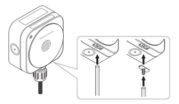
If the gas detector is installed in a difficult-to-access location, such as overhead on a ceiling, the remote gassing connection can be used to apply a test gas from a convenient location. Connect a tube appropriate for the type of gas being detected to the gas detector for bump test.
