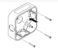
Secure the back box in its mounting position with suitable fixings appropriate to the mounting surface.
