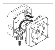
2. Remove the detector module of Sensepoint XCL.
