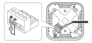
If an external power source is used, make sure that the fourth terminal is properly grounded for the analog output.
