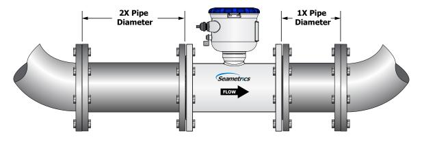
Minimal straight pipe requirements, in most cases, to ease installation in tight quarters.
