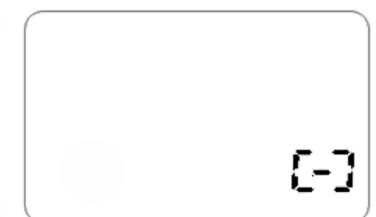
Meter Installed Backwards
