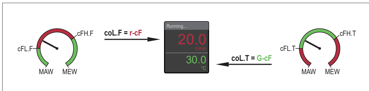
Fig. 21: Colour change. Example: coL.F = r-cF ; coL.T = G-cF ; current measured values between the limit values.
