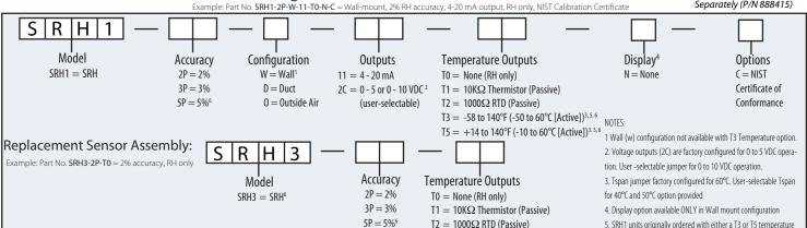
$T3 = -58 \text{ to } 140^{\circ}\text{F} (-50 \text{ to } 60^{\circ}\text{C [Active]})^{5}$
