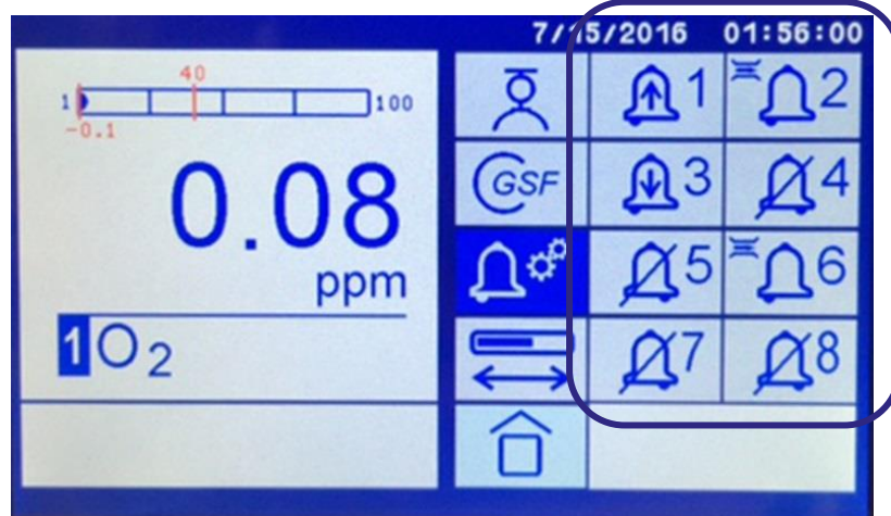
Figure 5-18: Alarms screen showing 8 alarms which have been set
