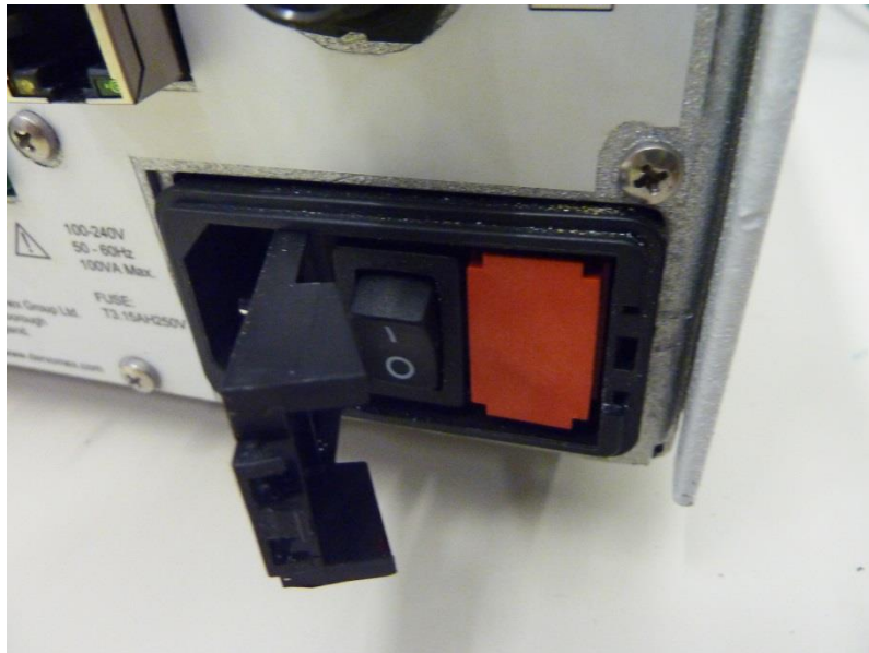
Figure 10-2: Fuse panel opened
