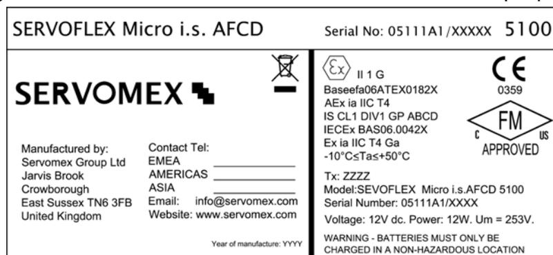
Figure 5 - Certification label: 5100S-Series with AFCD
