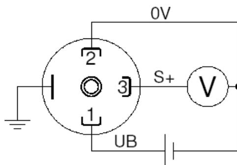
The transmitter metal case should always be connected to ground (GND) through the process connection thread in order to protect the sensor from disturbances due to electromagnetic fields or electrostatic charges.
