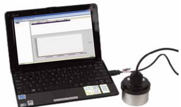
Sensor cap connected to laptop via calibration cable.
