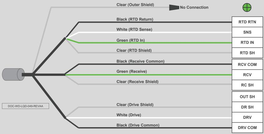
Clear outer shield wire is present in high temperature sensor options only
