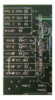
Figure 3-6 pH/ORP/ISE Signal Board and Sensor Cable Leads
