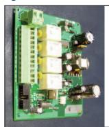
This power supply automatically detects DC power and accepts 20 Vdc to 30 Vdc inputs. Four programmable alarm relays are included.
