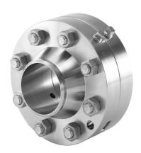
Standard flange styles are RF weld neck, RF slip-on, or RF threaded for paddle type orifice plates, and ring type joint RTJ weld neck for universal type plates with plate holders. All flange unions are supplied with studs, nuts, jackscrews, gaskets, and pipe plugs.
