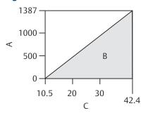
Maximum Loop Resistance = 43.5 × (Power Supply Voltage – 10.5)
