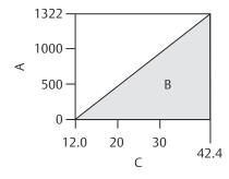
Maximum Loop Resistance = 43.5 × (Power Supply Voltage – 12.0)
