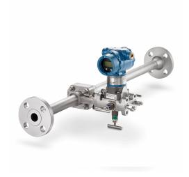
Rosemount 3051CFP Integral Orifice Flow Meters enable highly accurate flow measurement in small line sizes. Internal pipe diameter variation in combination with plate centering issues can greatly magnify flow measurement errors in small line sizes. Integral Orifice Flow Meters use a precision honed pipe section to minimize internal pipe diameter variation along with a self-centering plate design to eliminate alignment errors.
