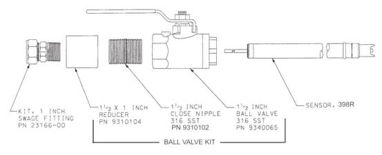
Ball Valve Kit includes 1-1/2 in. x 1 in. reducer, 1-1/2 in. close nipple, and 1-1/2 in. ball valve]
