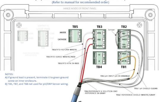
Wiring the Rosemount 398R/398RVP Sensor
