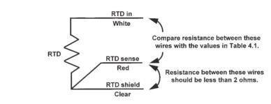
Consult Table 6.1 (above) for temperature-resistance data. Lead resistance is about 0.05 ohm/ft at 25°C. Therefore, 15 ft of cable increases the resistance by about 1.5 ohm. The resistance between the RTD return and RTD sense leads should be less than 2 ohms. If a connection is open or shorted and should not be, replace the sensor. If the measured resistance is greatly in error, replace the sensor.
