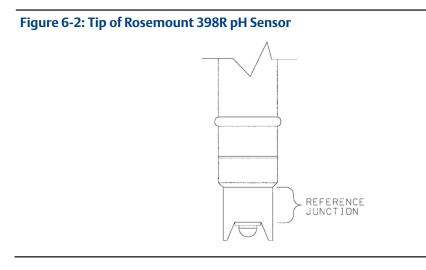
The figure shows the tip of the Rosemount 398R pH sensor. The bottom of the liquid junction is about even with the top of the wings that form the slotted tip. Keep acidic and alkaline solvents away from the liquid junction. If acids or bases get into the junction, subsequent pH readings may drift for several hours.
