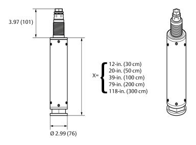
Figure 5. Accessories - Neck Extension for High Temperature (Process Operating Temperature Code H)
