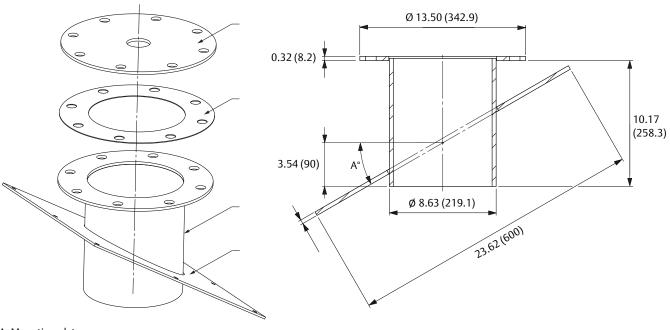
A. Mounting plate B. Gasket C. Adapter tube
