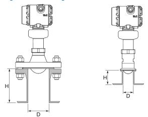
**Table 19: Nozzle Requirements for Process Seal Antenna**
