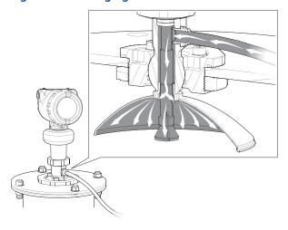
An air purge connection is also available for cone antennas with flanged connection by selecting option code PC1. This option consists of an antenna with purge holes and a separate air purge ring (see Figure 14).
