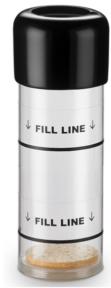
Figure 3-3: Fill the calibration chamber to the upper fill line with fresh sodium sulfite solution
