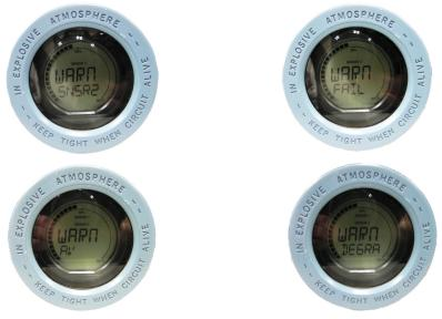
After the sensor has been repaired or replaced, the LCD display warning message will clear and display the output of the primary variable.
