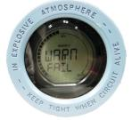
After the sensor has been repaired or replaced, the LCD display warning message will clear and display the output of the primary variable.
