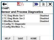
6. Select the sensor for which Thermocouple Diagnostic will be configured. Select from **1 Sensor 1** or **2 Sensor 2** and select **ENTER**. Select **3 Exit** to exit the setup.
