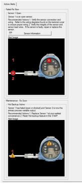
After the sensor has been repaired or replaced, the device status in the Process Variable Overview section of the DTM will change from Failed to Maintenance.
