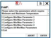
7. Select which variable to track with the selected parameter. Select between Sensor 1, Sensor 2, Average Temperature, First Good Temperature, Differential Temperature, and Terminal Temperature. Select ENTER.
