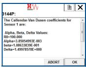
8. Select which set of CVD coefficients you would like to enter for that sensor. Select between 1 R0, A, B, C, and 2 R0, Alpha, Beta, Delta.
