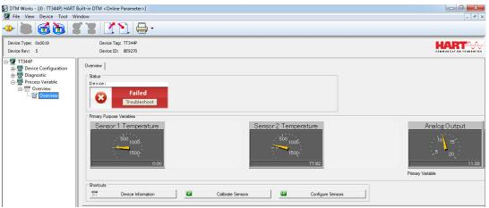
To investigate why the device displays a Failed status, select **Troubleshoot** in the red device status box. Another screen will display the active alerts indicating *FAILED Sensor 1 Open*, and *MAINTENANCE Hot Backup Active*, as shown below:
