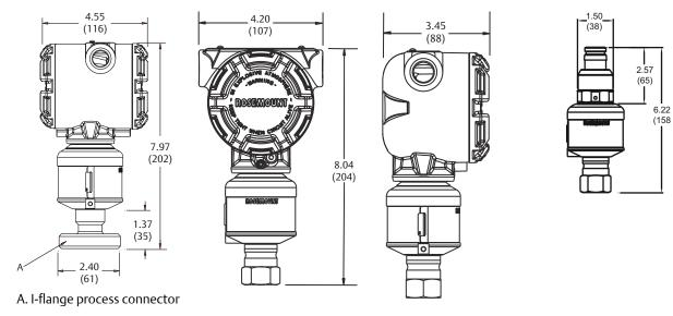
Figure 10: Plantweb Housing, Junction Box Housing, and Quick Connect with In-line SuperModule<sup>™</sup> Platform
