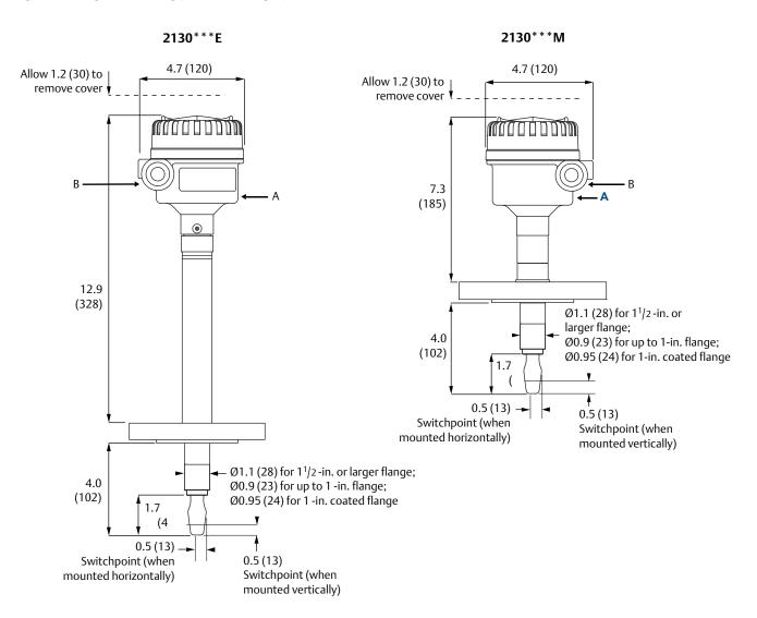
A. Aluminum or stainless steel housing B. Cable entry M20 x 1.5 or  $^{3}/_{4}$ -in. ANPT
