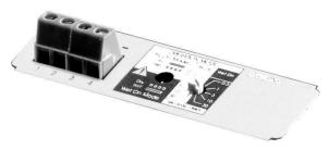
There is a variety of plug-in electronics options, with each having an adjustable mode and switching delay (see "Electrical" on page 11)
