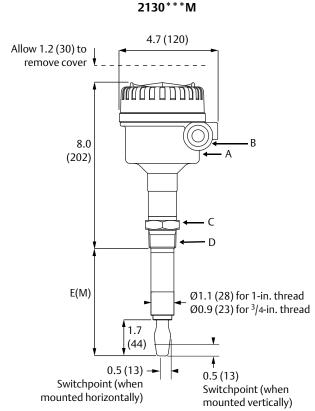
A. Aluminum or stainless steel housing B. Cable entry M20 x 1.5 or  $^{3}/_{4}$ -in. ANPT
