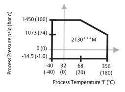
**Figure 2. Operating Temperatures**
