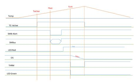
Note: Thermal Zone 'Active' is optional and not implemented in the RXi2-BP fanless design.
