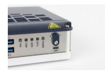
5. To remove the  $\mu$ SD card, remove the lid first and push it carefully in the same direction as step 3, the  $\mu$ SD card will pop out slightly and can then be removed.
