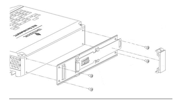
There are two DIN rail mounting options available, depending on the size of the DIN rail connector.
