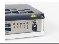
4. Re-attach the lid and tighten the screw to 0.45 Nm (Figure 12).
