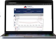
access from any location. Data is transmitted from wireless data loggers directly to the RFC1000 Cloud Relay and relayed to the MadgeTech Cloud. From there, it can be viewed on any internet enabled device such as a computer, tablet, smartphone or other mobile device.
