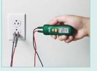
Take voltage measurements using the attachable test lead tip
